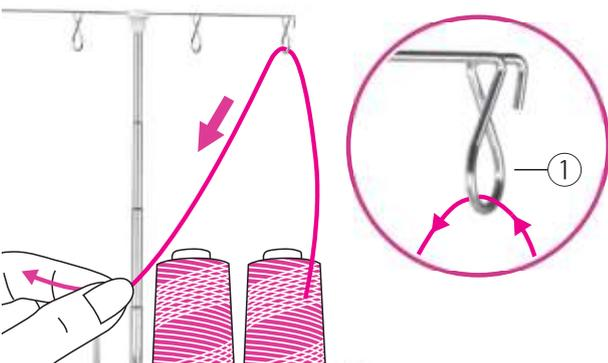
Pull the thread and pass it through the thread guide on the thread stand from back to front and pull down.
