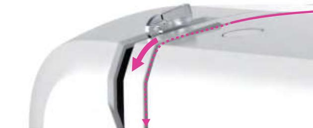
5. Continue to guide the thread into the silver discs to keep the thread in proper tension.
