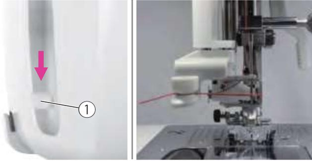
11. Press down the automatic needle threader lever on the left side of face cover to the bottom, when you hear a "click" sound, it is the correct position and the hook pin passes through the needle eye.
