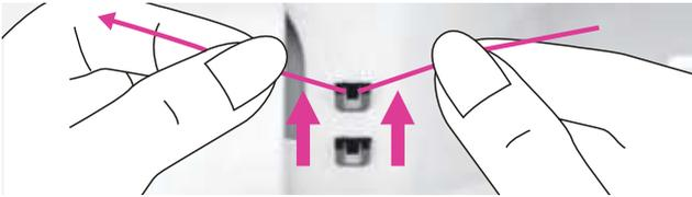
3. Draw the thread from the spool and place the thread in between the upper thread guide.
