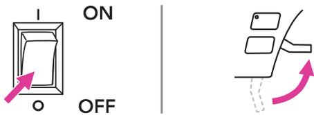
Turn the power switch to off ("O"). Raise the presser foot lifter.
