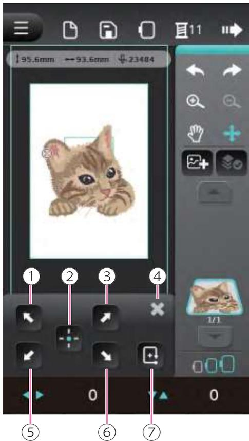
Use the center of the pattern as the alignment reference point.
