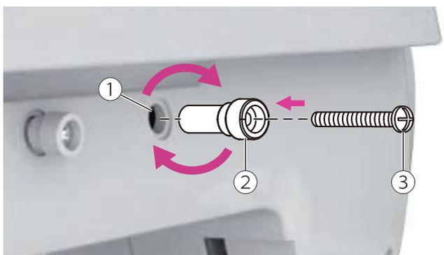
Take out the screws and screw holders from the accessories bag, screws has to be inserted through the screw holders. Then insert the 3 screw holders with screws into the holes and tight it clockwise.
