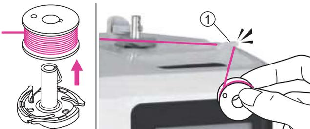
8. Remove the bobbin then use the thread cutter on the right side to cut.
