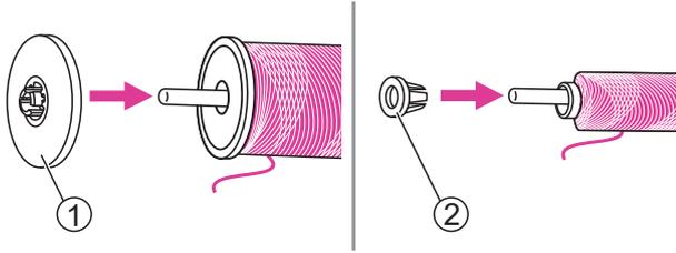
2. Place the thread and spool holder onto the spool pin. For better sewing quality, choose a proper size of the spool holder for the thread and attach it next to the thread.
