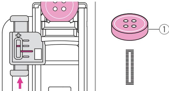
The buttonhole length may need to be increased for thick button, adjust the pointer toward to "+" for fine tuning.
