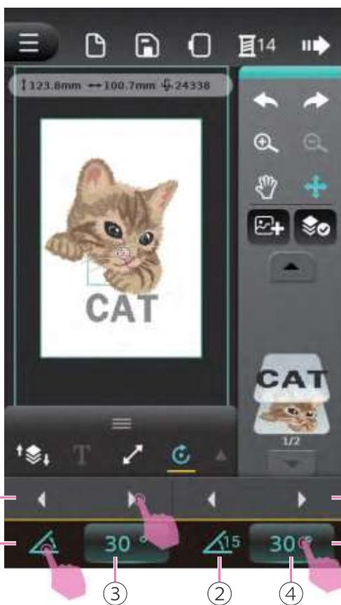
Preview screen will display the rotated patterns. The default value is 0, click Angle icon to display multifunction list. The left and right icon can adjust the angle clockwise or counterclockwise.
