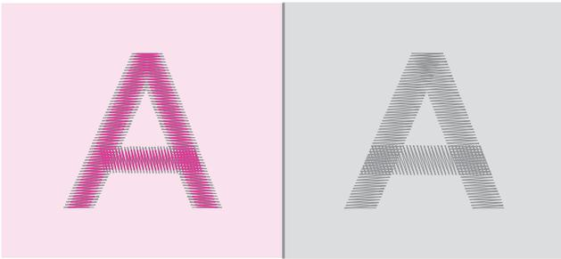
When the bobbin thread is visible on the front of the fabric, the thread tension is too tight for embroidering. To reduce the tension, press the "-" button.
