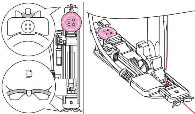
Attach the electronic buttonhole foot and plug the cord into the socket above the presser foot bar. Bring the gimp thread ends to the front of the foot and insert them into the grooves, then tie them there temporarily. Lower the presser foot lifter and start sewing.
