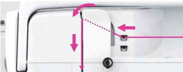
Guide the thread to the left and pass through the guide plate.
