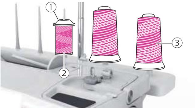
There are 5 spool pins. Two of the right side are for larger threads and three of the left side are for small threads.
