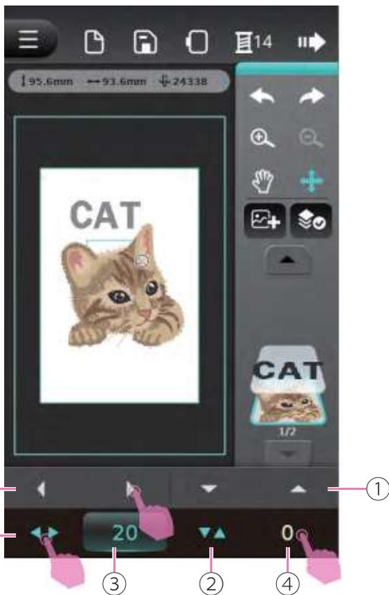
Click Direction icon to display multifunction list. The default value is 0. The left and right, up and down icon can adjust X-axis and Y-axis position.
