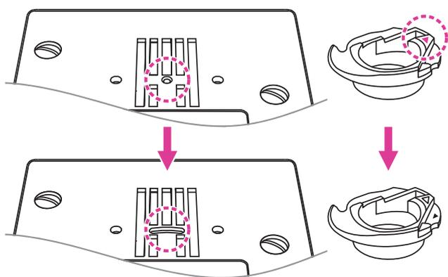
Replacing the straight stitch needle plate to normal needle plate.
