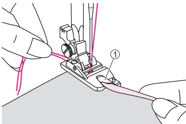
Insert the needle into the fold by turning the handwheel toward you, and lower the presser foot lifter. Sew several stitches and raise the presser foot lifter.
