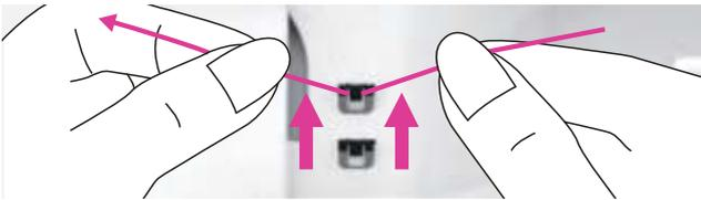
Guide the thread forward and pass through upper thread guide.
