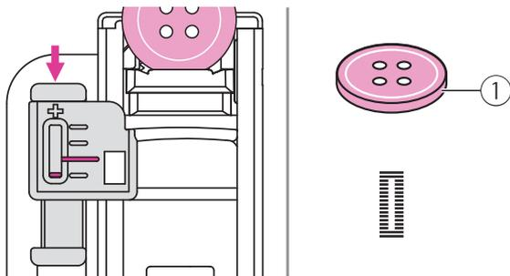
The buttonhole length may need to be decreased for thin button, adjust the pointer toward to "-" for fine tuning.
