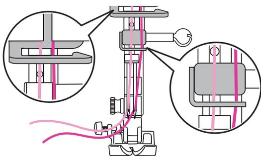
As shown in the picture, pull the thread from the horizontal spool holder pass through left needle hole manually and thread from the second spool holder pass through right needle hole.
