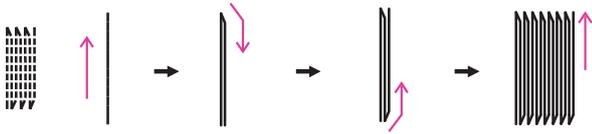
Darning stitches are sewn from the front of the presser foot to the back, as shown.
