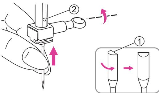
Inserting a proper needle, keep the flat side of the shaft to the back.
