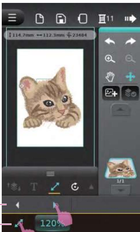
Preview screen will display the adjusted patterns. The default value is 100%. Click Lock aspect ratio icon to display multifunction list. The left and right arrow icon can scaling the pattern size with the fixed proportion.
