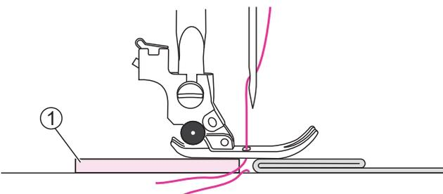
You also can place another piece of fabric with the same thickness at the back of the seam. Or support the presser foot while feeding by hand and sewing toward the folded side.
