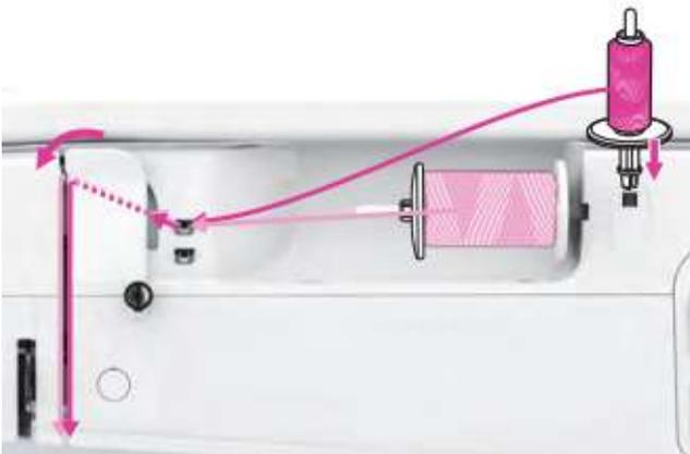
Set the second spool pin into the hole on the top of the machine and put spool pin felt and thread onto second spool holder.
