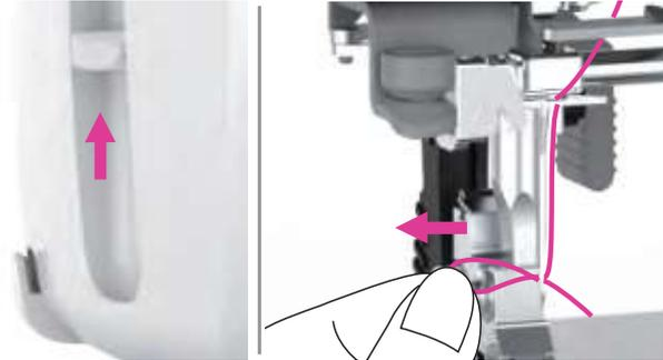
12. Raise the lever, the hook will rotate and pass the thread through the needle eye to form a loop.
