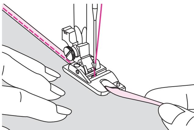
Lower the presser foot lifter and start sewing slowly guiding the raw edge of the fabric in front of the hemmer foot evenly into the scroll of the foot.
