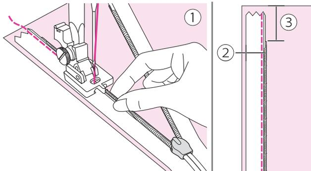
Attach the invisible zipper foot to the machine, with the needle lined up with center mark. Place open zipper face-down on right side of fabric as shown. Pin in place with coil on seam line (1.6 cm) and top stop 1.9 cm below raw edge of garment. With right-hand groove of foot over coil, stitch zipper until the foot hits the slider (remove pins as you come to them.) Back-tack.
