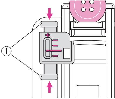
Consider the shape and height of each button, buttonhole fine tuning adjuster provides fine adjustment of the buttonhole length.
