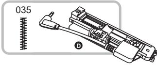
Using the electronic buttonhole foot.
