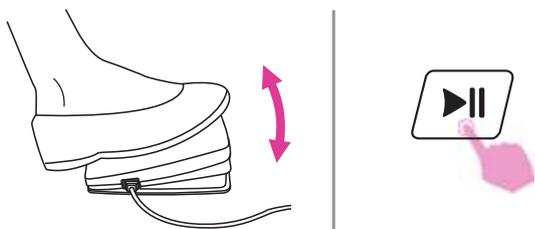
4. Slowly press down the foot control or long press the start/stop button to start sewing, presser foot will automatically lower at the same time.
