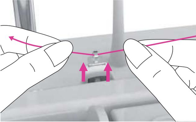
Pass the thread through the thread guide on the spool base.
