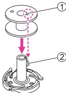
4. Place the empty bobbin on the bobbin winder spindle. Then align the notch with bobbin winder spindle spring.
