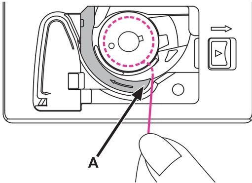
Pull the thread through the slit (A).
