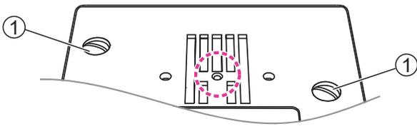
Change the straight stitch plate and tighten the screws.
