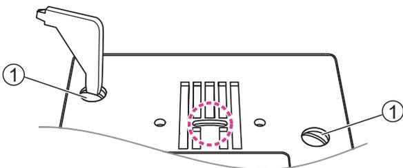
Remove the screws on the needle plate then remove the needle plate.
