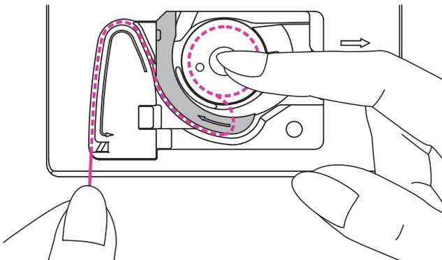
With a finger hold gently on top of the bobbin, please follow the arrow markings and draw the thread into the bobbin thread guide.
