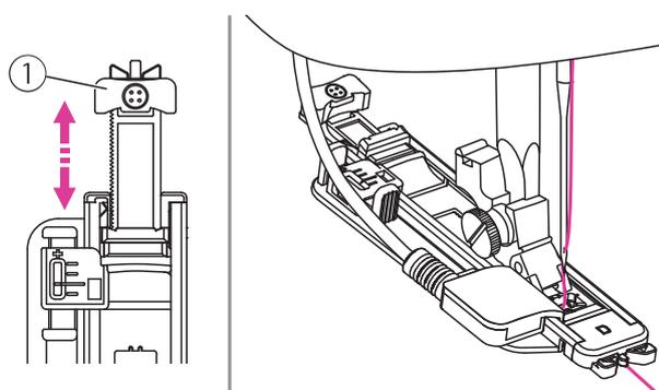
Extend the button holder plate and set to the desired length. Adjust the stitch width and the stitch length to the desired width and density.
