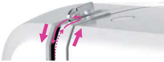
7. Pull the thread to the top then pass the thread through the slotted eye of the take-up lever. Guide the thread down afterwards.
