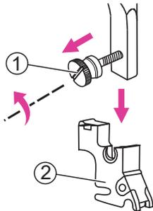
Loosen the screw counter-clockwise to remove the presser foot holder.
