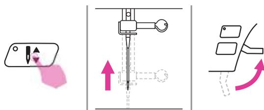
5. Press the needle up/down position button to raise the needle. Raise the presser foot lifter and remove the fabric.
