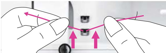
2. Draw the thread from the spool and place the thread in between the bobbin thread guide.
