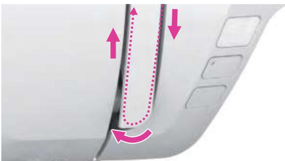
6. Pass the thread under the take-up spring then pull it upwards as arrow marks illustrated.
