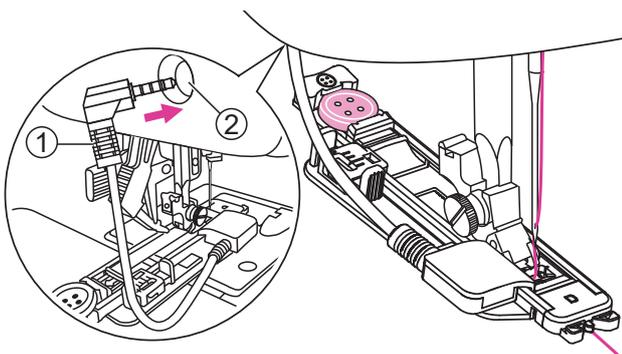
Attach the electronic buttonhole foot and plug the cord into the socket behind the face cover.
