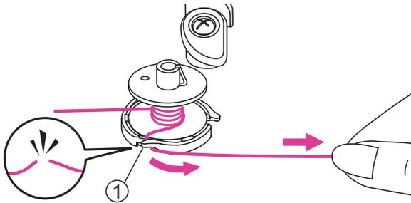
6. Wind the thread into the cutter of bobbin winder base and pull the thread to the right to cut.
