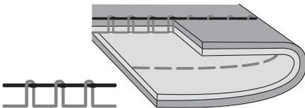
Thread tension is too tight for straight stitch sewing. Turn the dial to the lower number.
