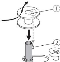
4. Place the thread end through one of the inner holes as illustrated and place the empty bobbin on the bobbin winder spindle. Then align the notch with bobbin winder spindle spring.
