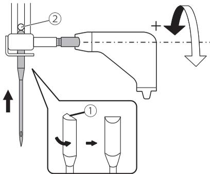
When inserting a new needle, keep the flat side of the shaft to the back.
