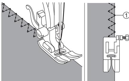
Sewing the overcasting along the edge of the fabric so that the needle drops over the edge of the fabric on the right side.
