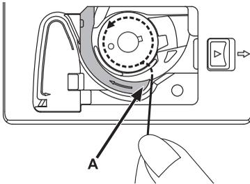
Pull the thread through the slit (A).
