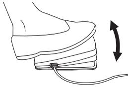
7. Slowly press down the foot control to start sewing. Release the foot control to stop the machine.
