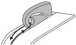
8. Pull the thread to the top then pass the thread through the slotted eye of the take-up lever. Guide the thread down afterwards.
