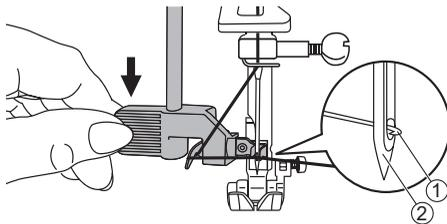
12. The needle threader automatically turns to the threading position and the hook pin passes through the needle eye.
