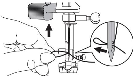
14. Hold the thread loosely and release the lever slowly. The hook turns and passes the thread through the needle eye forming a loop.
