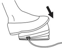
7. Step on the foot control to start winding the bobbin.
