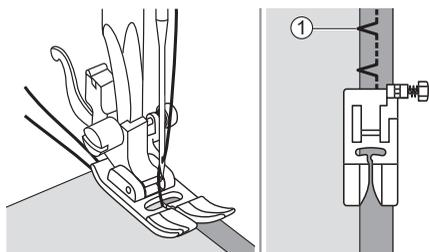
Place the fabric under the foot. Turn the handwheel forwards until the needle swings fully to the left. It should just pierce the fold of the fabric.
