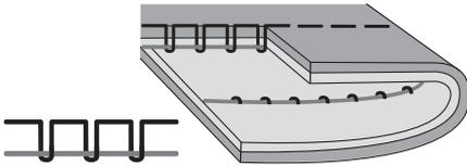
Thread tension is too loose for straight stitch sewing. Turn the dial to the higher number.
