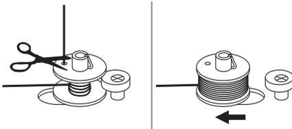
8. After the bobbin has wound a few rounds, stop the machine and cut the thread near the hole of the bobbin. Continue filling the bobbin until it is full. Once the bobbin is full, it rotates slowly. Release the foot control to stop the machine, then push the bobbin winder spindle to the left.
