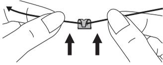
4. Draw the thread from the spool and place the thread in between the thread guide.
