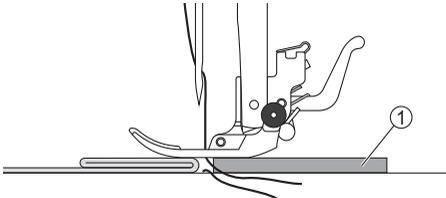
You can place cardboard or thick fabric with the same thickness at the back of the seam. Or support the presser foot while feeding by hand and sewing toward the folded side.
