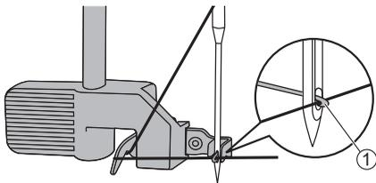
13. Take the thread in front of the needle and make sure it is under the hook pin.
