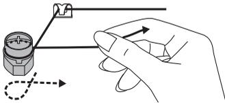
3. Wind the thread clockwise around the tension discs.
