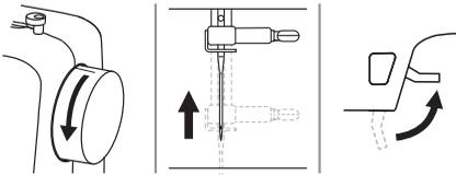
8. Turn the handwheel toward you (counterclockwise) to raise the needle. Raise the presser foot lifter and remove the fabric.
