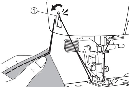
9. Guide both threads to the side of the face plate and into the thread cutter. Pull the threads down to cut them.
