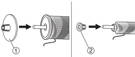
3. Place the thread and spool holder onto the spool pin. For better sewing quality, choose a proper size of the spool holder for the thread and attach it next to the thread.
