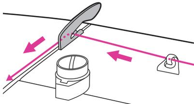
5. Guide the thread ahead and pull the thread through the pre-tension spring as illustrated.
