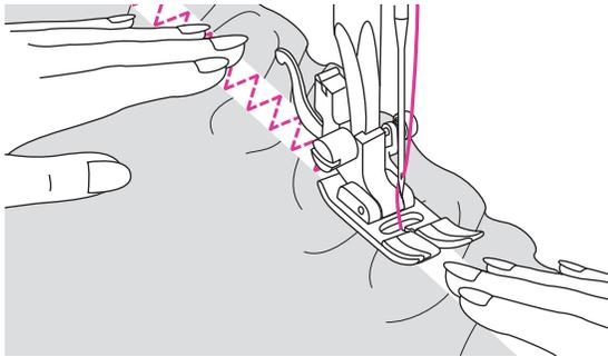
Sew the elastic tape to the fabric while stretching the tape so that it is the same length as the fabric.
