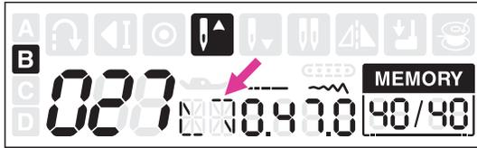
Under the memory program, the reverse button is using for repeat sewing. The stitch combination can be sewn continuously if the icon appeared.
