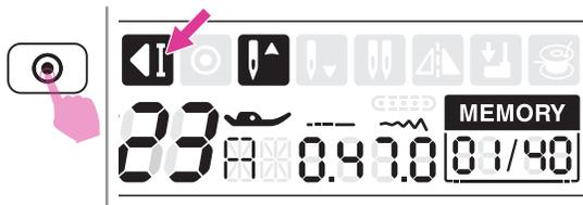
During machine is sewing, the machine will sew 3 locking stitches at the end of the current stitch if the auto-lock button pressed. Then it will stop automatically. The LCD screen will display the auto-lock icon. If pressing the start/stop button again, it will sew from the next stitch.
