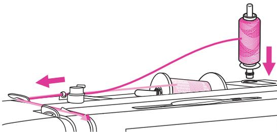
Follow the instructions for single-needle threading using the horizontal spool pin. Thread through the left needle.
