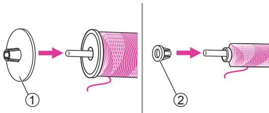
1. Place the thread and spool holder onto the spool pin. For better sewing quality, choose a proper size of the spool holder for the thread and attach it next to the spool.
