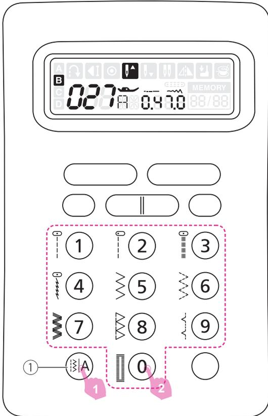
The LCD screen will be set at A-Direct Pattern Group. By pressing the pattern group switch button to select the stitch mode.
