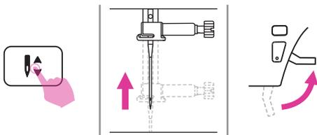
8. Press the needle up/down position button to raise the needle. Raise the presser foot lifter and remove the fabric.
