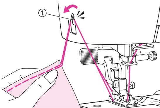
9. Guide both threads to the side of the face plate and into the thread cutter to cut them.
