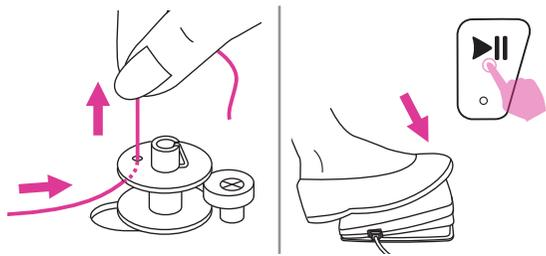
6. Hold the thread tail securely in one hand. Step on the foot control or press the start/stop button to start winding the bobbin.
