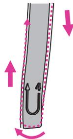
7. Pass the thread under the take-up spring then pull it upwards as arrow marks illustrated.
