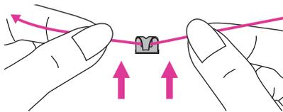
2. Draw the thread from the spool and place the thread in between the upper thread guide.
