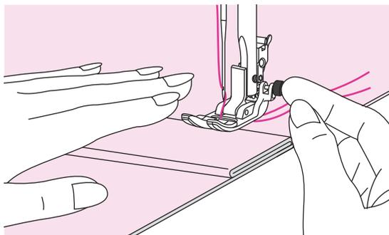
When you reach the point of an increased thickness, lower the needle and raise the presser foot lifter. Press the toe of the foot to the horizontal line and push in the black button, then lower the foot and continue sewing.
