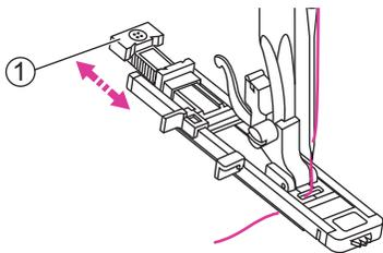
Extend the button holder plate and set to the desired length. Adjust the stitch width and the stitch length to the desired width and density.
