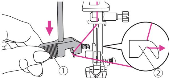
11. Lower the needle threader lever slowly and draw the thread through the thread guide as illustrated and then to the right.
