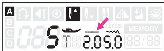
Press the stitch length adjustment button "+" or "-" to adjust the stitch length. Neat zigzag stitches are usually achieved at "2.5" or below.
