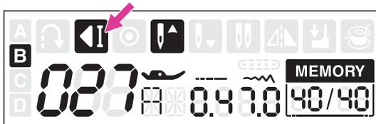
Press the reverse button to cancel the repeat sewing, machine will sew 3 locking stitches at the end of one complete combination. The LCD screen will display the auto-stop icon during sewing the last stitch.
