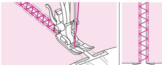
Align the center of the presser foot with the center of the two pieces of fabric and begin sewing.
