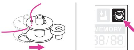
5. Push the bobbin to the right. When the bobbin winder spindle is pushed to the right, the screen will display the figure.
