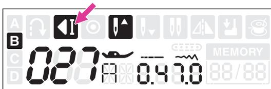
During machine is sewing: When A-Direct Pattern Group number 6-9 or B-Regular Pattern Group number 001-007 or 021-105 is selected, the machine will sew 3 locking stitches at the end of the current stitch if the auto-lock button pressed. Then it will stop automatically. The function can be cancelled if pressed the button once again during sewing.
