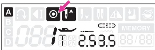
When machine is not sewing: Press the auto lock button, machine will sew 3 stitches in the same position then stop.
