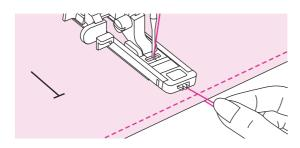
Slightly hold the end of the upper thread and start sewing. Pull two lines together.
