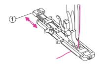
Extend the button holder plate and set to the desire length. Adjust the stitch width and the stitch length to the desired width and density.
