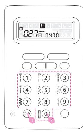
The LCD screen will be set at A-Direct Pattern Group. By pressing the pattern group switch button to select the stitch mode.
