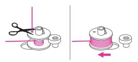
7. After the bobbin has wound a few rounds, stop the machine and cut the thread near the hole of the bobbin. Continue filling the bobbin until it is full. Once the bobbin is full, it rotates slowly. Release the foot control or press the start/stop button to stop the machine, then push the bobbin winder spindle to the left.
