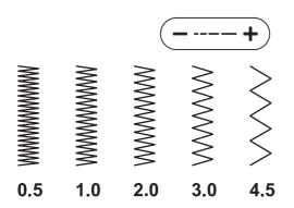
Press the stitch length adjustment button "+" or "-" to adjust the stitch length. Neat zigzag stitches are usually achieved at "2.5" or below.
