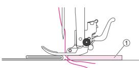
You also can place another piece of fabric with the same thickness at the back of the seam. Or support the presser foot while feeding by hand and sewing toward the folded side.
