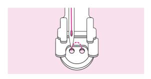
Select the buttonhole sewing stitch and adjust the stitch width according to the distance between the two holes of the button.
