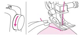
Turn the handwheel toward you (counterclockwise) to lower the needle into the fabric at the beginning of the stitching.
