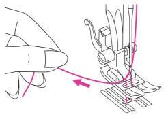
Gently pull on the upper thread to bring the bobbin thread up through the needle plate hole. The bobbin thread will come up in a loop.
