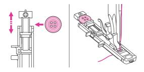
Pull the button holder plate to the back, and place the button in it. Push back the button holder plate against the button to hold it tight.
