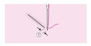
Position the fabric so that the needle is 2mm in front of the area to be darned, and then lower the presser foot lifter.
