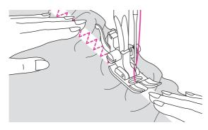
Sew the elastic tape to the fabric while stretching the tape so that it is the same length as the fabric.
